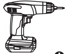
Electric Screwdriver + Torque set to 3-5
