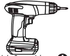
Electric Screwdriver ⊕ Torque set to 3-5
