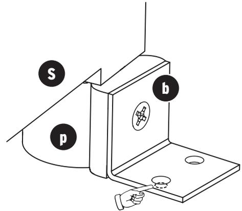
Align one hole with pre-drilled hole
