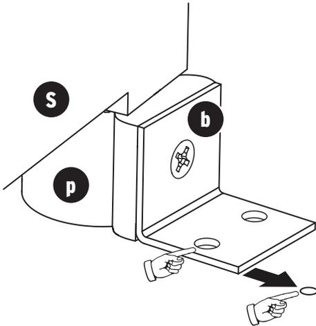
Slide **S Support Leg** with **b/p Plastic Support Tube Assembly** to pre-drilled hole
