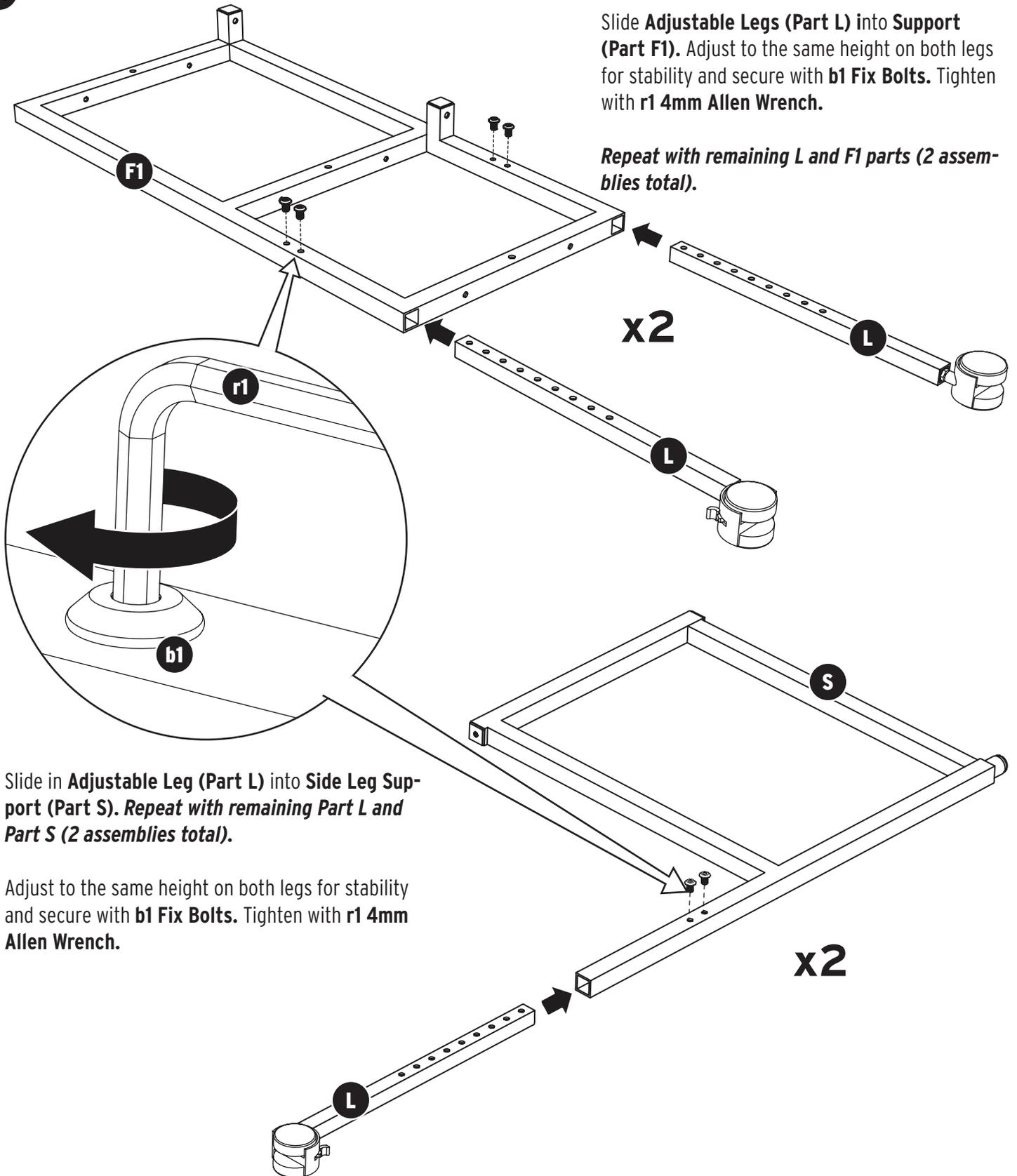
Slide **Adjustable Legs (Part L)** into **Support (Part F1)**. Adjust to the same height on both legs for stability and secure with **b1 Fix Bolts**. Tighten with **r1 4mm Allen Wrench**.
