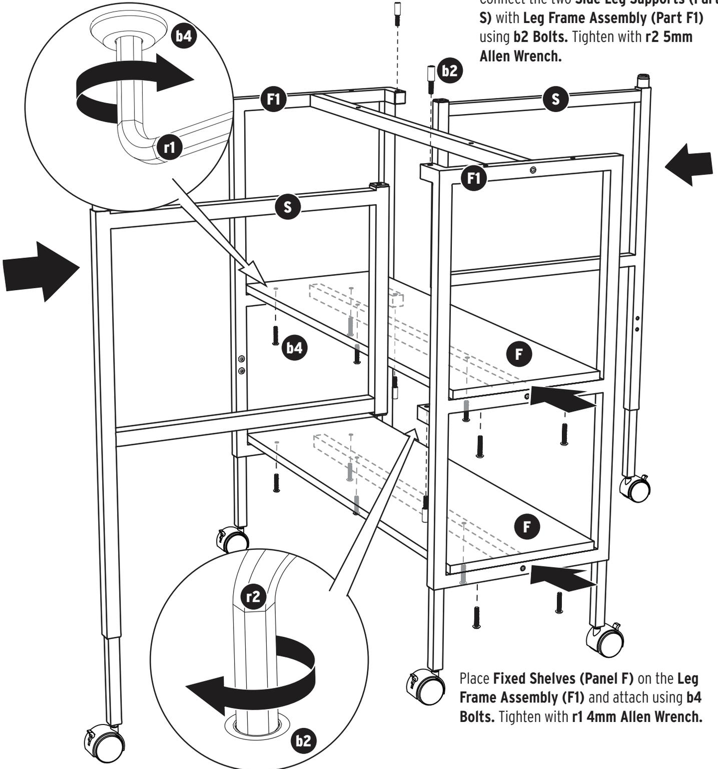
Place **Fixed Shelves (Panel F)** on the **Leg Frame Assembly (F1)** and attach using **b4 Bolts**. Tighten with **r1 4mm Allen Wrench**.
