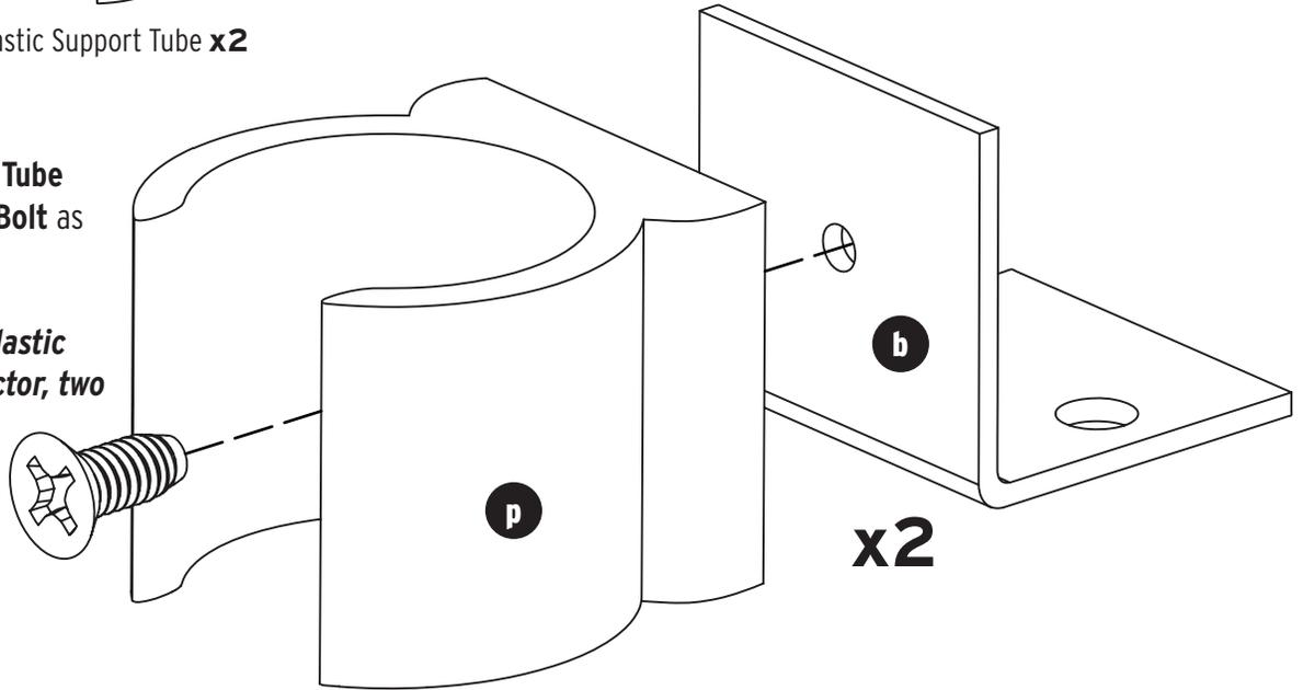
Click **b/p Plastic Support Tube Assembly** onto **S Side Leg Assembly**, as shown.
