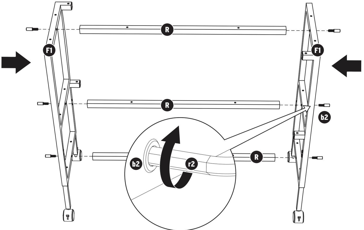
Connect the two **Frame Leg Supports (Part F1)** with three **Rails (Part R)** using **b2 Bolts**.
