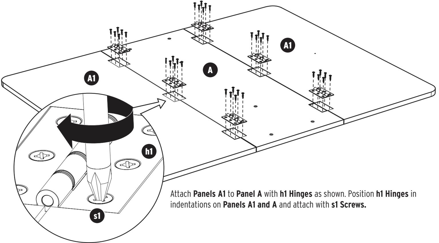
Attach **Panels A1** to **Panel A** with **h1 Hinges** as shown. Position **h1 Hinges** in indentations on **Panels A1** and **A** and attach with **s1 Screws**.
