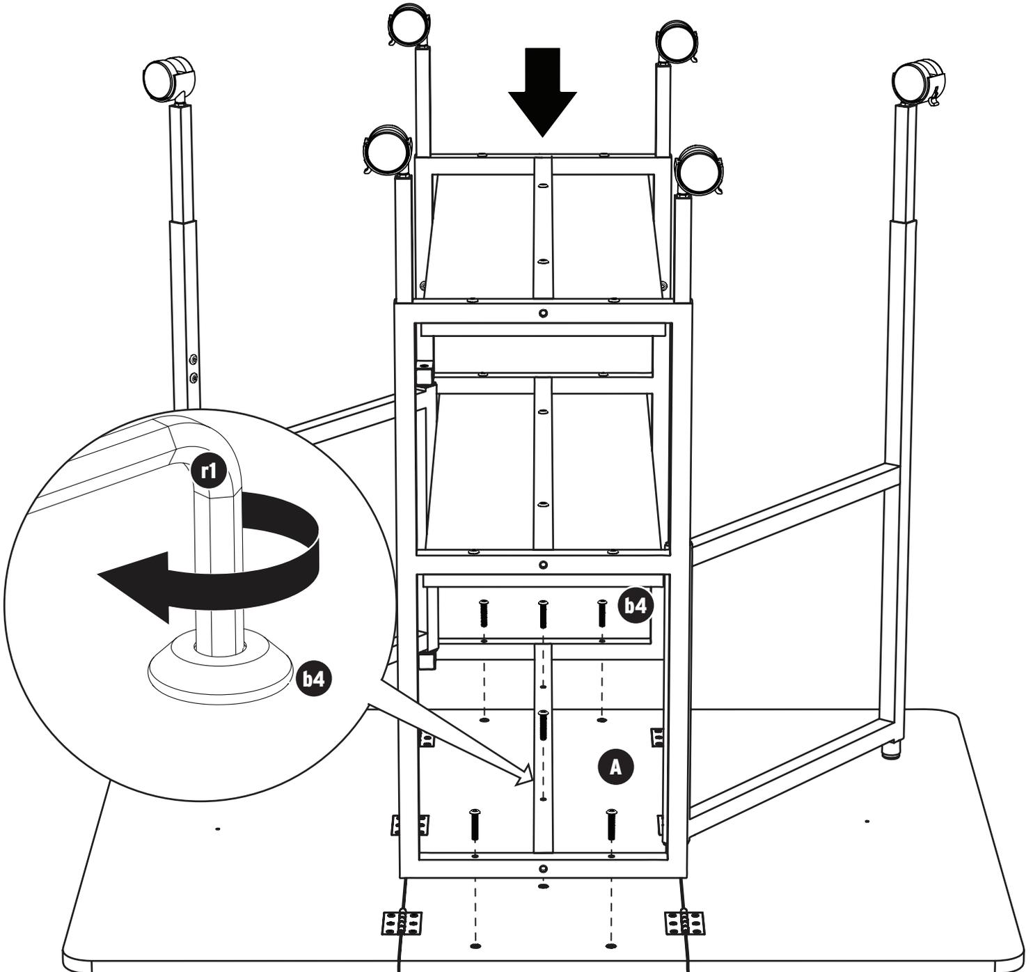
This step may require two people. Flip and align entire **Leg Assembly** with holes on **Panel A** and attach using **b4 Bolts**. Tighten with **r1 4mm Allen Wrench**.
