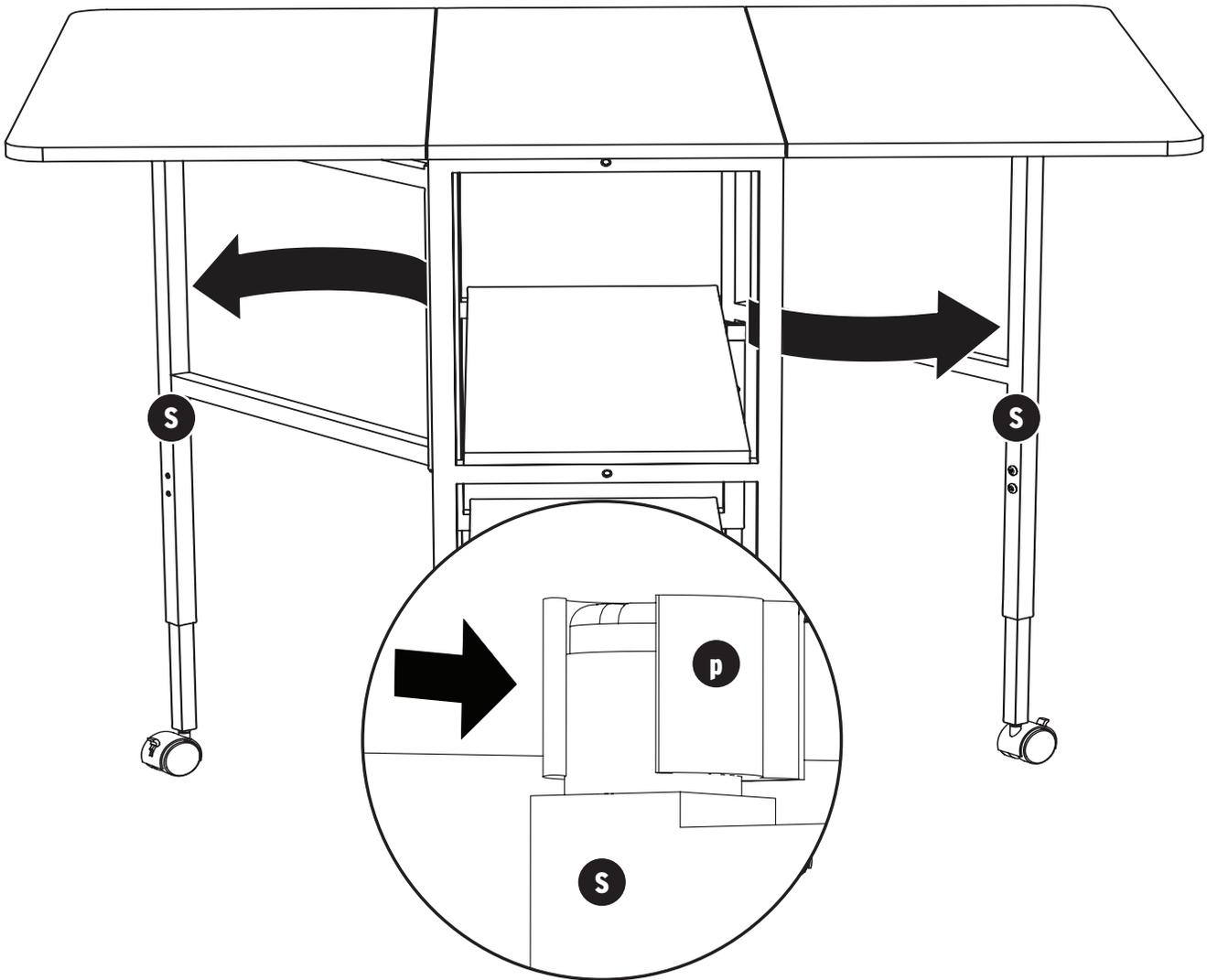
Make sure all legs contact the ground and side leg supports are properly snapped into connectors on both sides before use.
