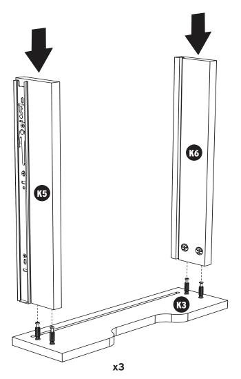
Attach side Panels K5 and K6 to drawer front Panel K3. Tighten cams and apply covers. Repeat x3
