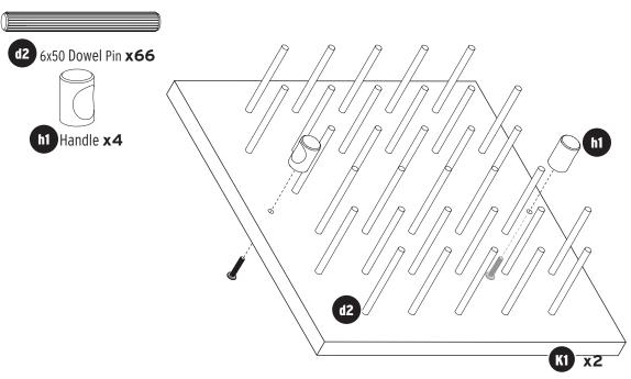
Insert d2 Dowel Pins into Panel K1. If you choose to use glue in this step, note that the dowels will not be reconfigureable once glue has set.
