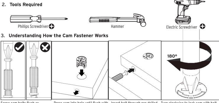
Screw cam bolts flush as illustrated.
