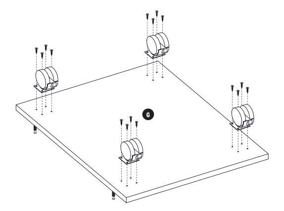
Turn the panel over and attach Plate Casters using s1 Screws.
