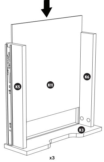
Slide drawer bottom **Panel K11** into the grooves on **Panels K5, K6 and K3.** *Repeat x3*
