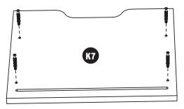
Prep drawer front  $\textbf{Panel}\ \textbf{K7}$  as shown above by installing 4  $\textbf{c1}\ \textbf{Cam}\ \textbf{Bolts}$
