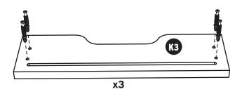
Prep drawer front **Panel K3** as shown above by installing 4 **c1 Cam Bolts.** *Repeat x3*
