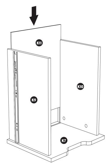
Slide drawer bottom **Panel K11** into the grooves on **Panels K9, K10 and K7.**
