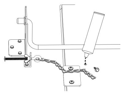
Place a few drops of wood glue or similar adhesive into the hole for the Hexagonal Bolt.
