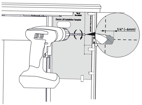
Drill pilot holes NO DEEPER THAN 1/4" into the panel.
