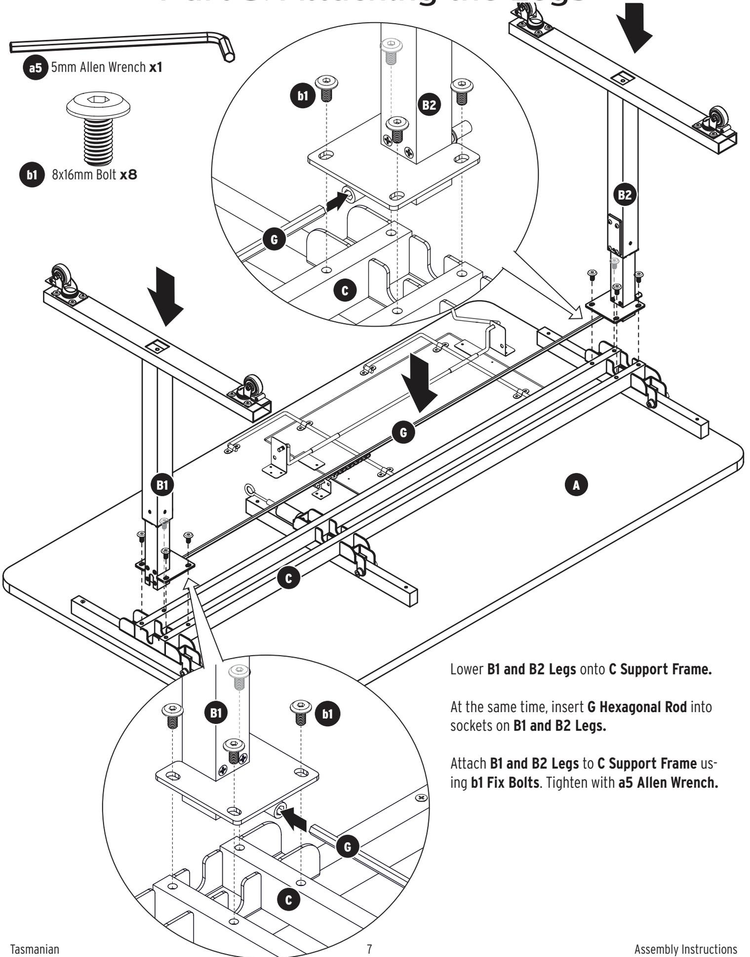
Lower **B1** and **B2** Legs onto **C** Support Frame.
