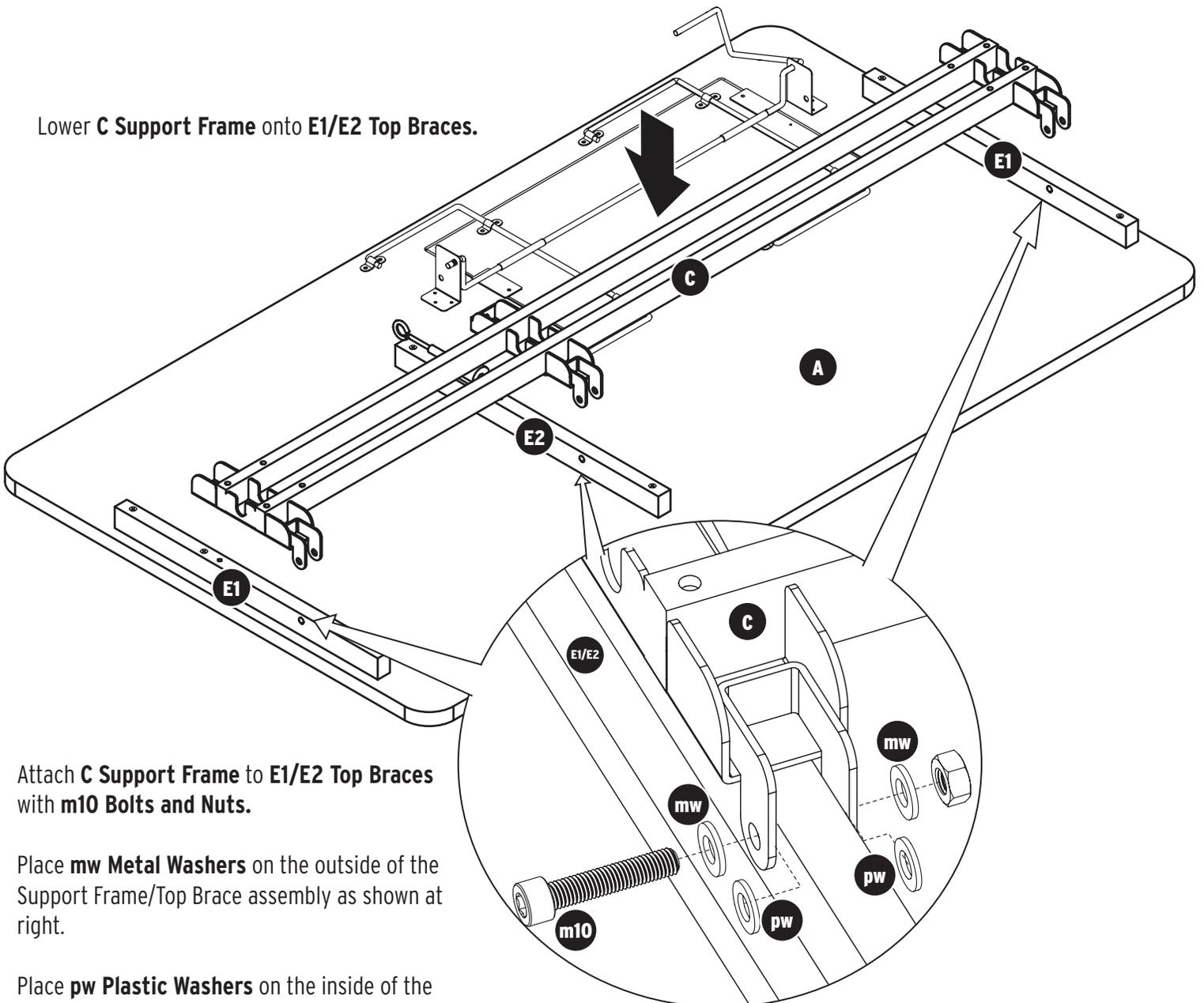
Attach **C** Support Frame to **E1/E2** Top Braces with **m10** Bolts and Nuts.
