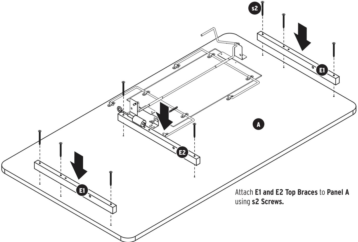
Attach **E1** and **E2** Top Braces to **Panel A** using **s2** Screws.
