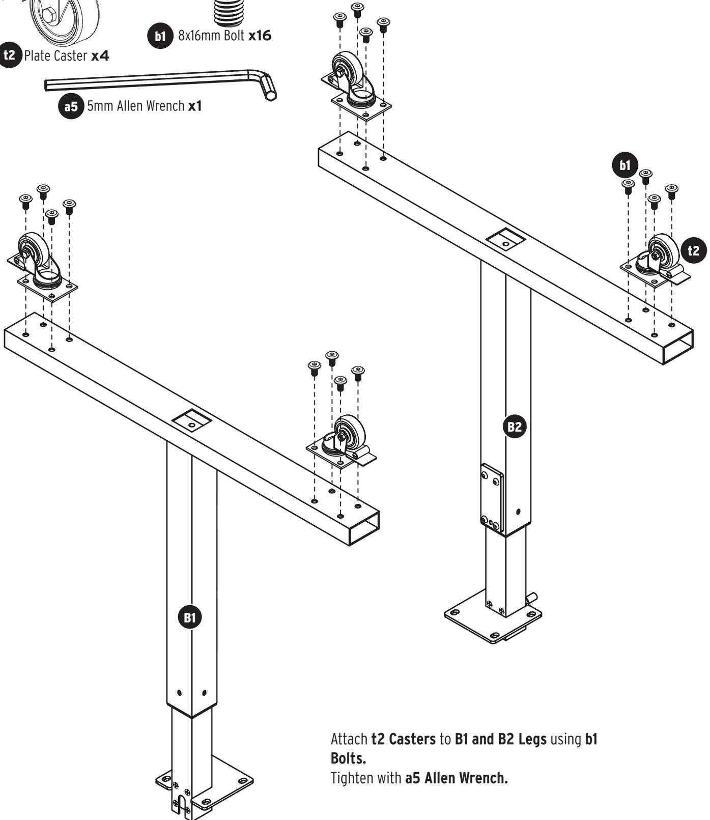
Attach **t2 Casters** to **B1 and B2 Legs** using **b1 Bolts**.
