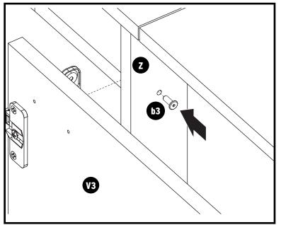
Insert female end of the **b3 Post Bolts** through the pre-drilled hole in **Panel Z**
