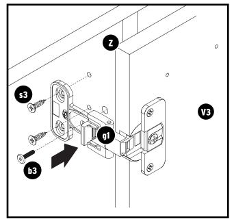
Attach **g1 Hinge Body** to **Panel Z** with 2 **s3 Screws.** Insert male end of the **b3 Post Bolts** through the **g1 Hinge Body** and tighten with one **a1 Allen Key** while holding the female end of the **b3 Post Bolt** stationary with the second **a1 Allen Key**
