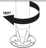
Screw cam bolts flush as illustrated.
